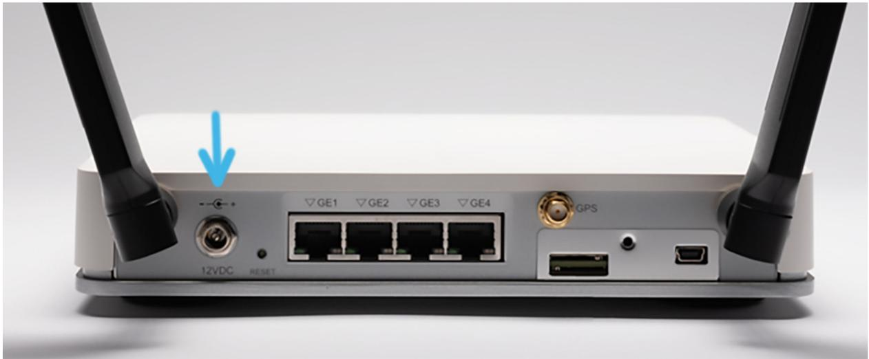
**Figure 3. Connect the power adapter to the AC power outlet**
